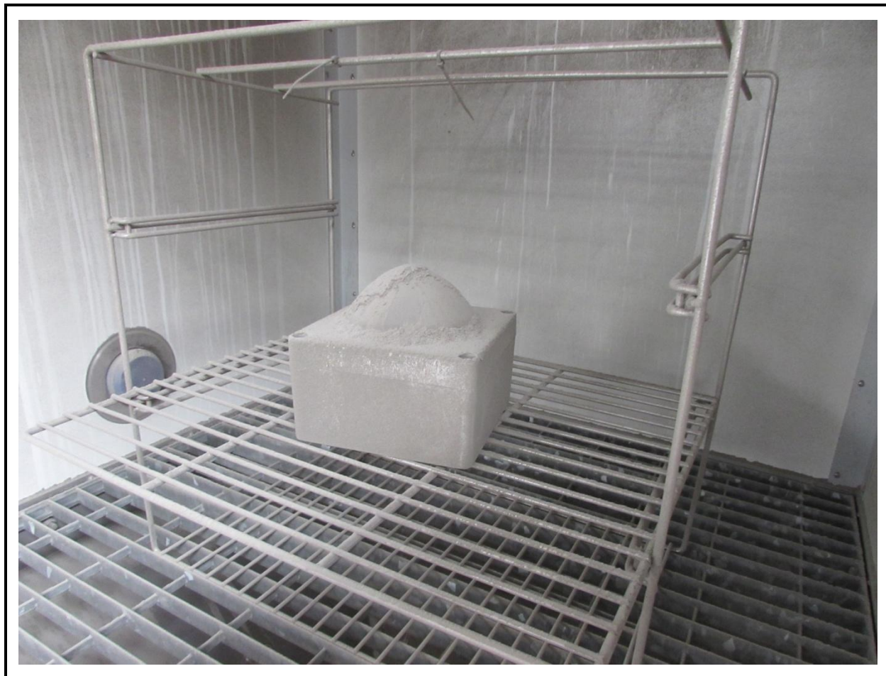
Figure 1: Test Item Mounting – IP6Kx Dust Ingress
